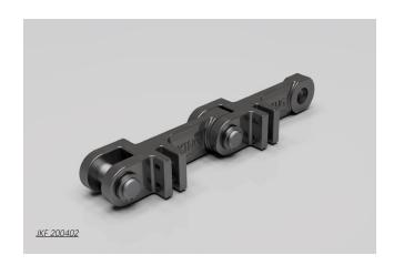
For double strand assemblies John King have a range of links following the standard format but with a forged "double clevis" into which a scraper can be mounted. The flight blade can be retained by either a U bolt or standard fasteners. The chain allows for some built in clearance between strands which obviates any potential problems that may be associated with mismatch. Double strand allows for improved discharge particularly relevant in conveying sticky materials.
