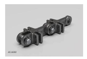
Where extra wide flights are required the John King triple link is available allowing, in conjunction with the double on perimeters, three chain strands up to 3100 mm overall. In addition the "Double slot" allows for a versatile means or flight retention for both steel & plastic options. Retention can be either U clips or standard fasteners.
